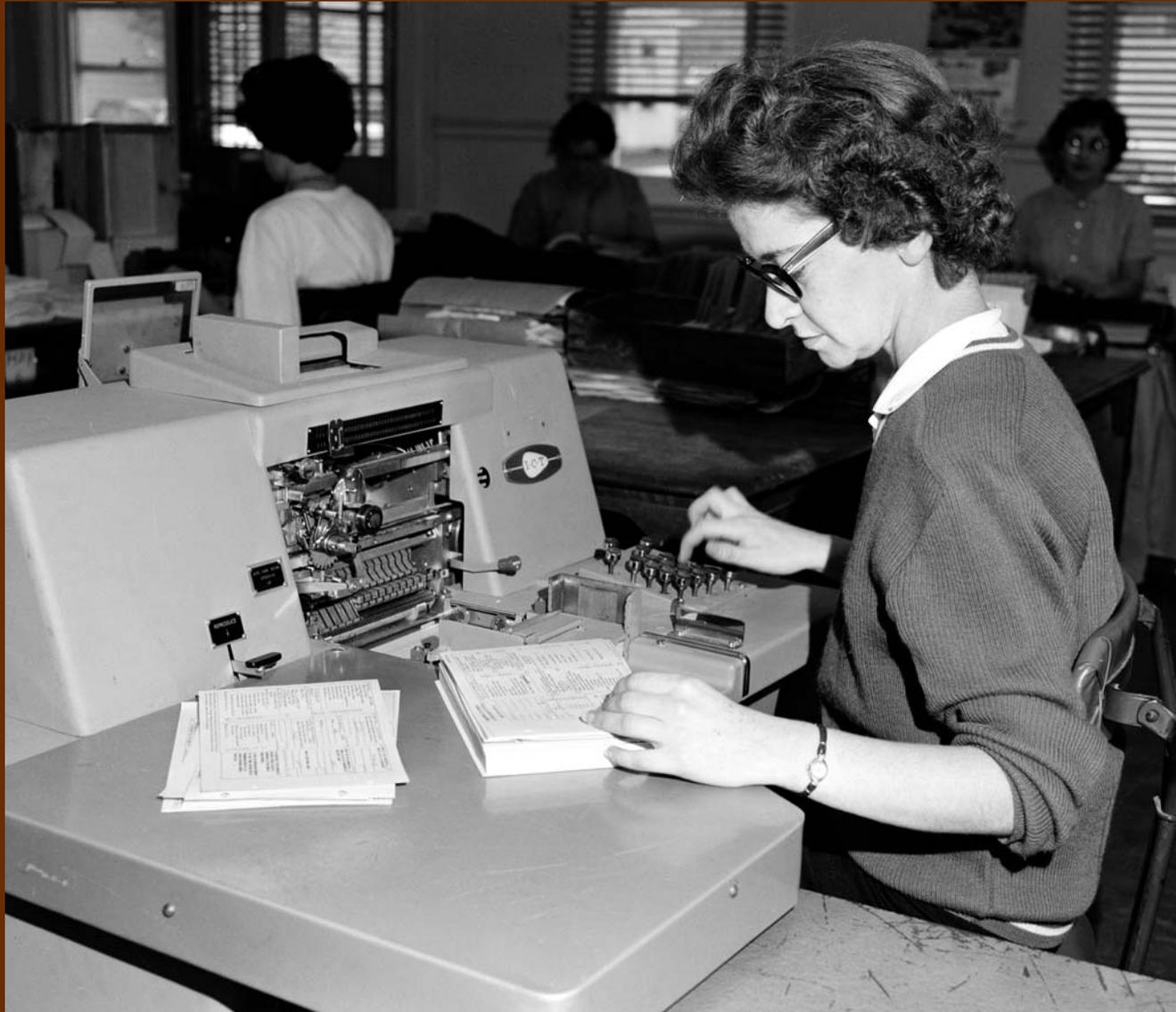
Operator of an ICT electric punch machine inputting respondent data from cards used in the labour force survey in the 1960s.
